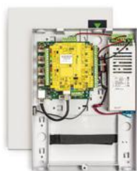
Entry - Control unit
