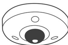
Fisheye cameras and Multi-Sensor cameras are unique in their capabilities – instead of pointing in a single direction, these cameras record video from multiple directions, covering up to a 360 degree view. Because of their view, they are often impossible to 'sneak up' on, and their lens can be protected by vandal resistant glass.
