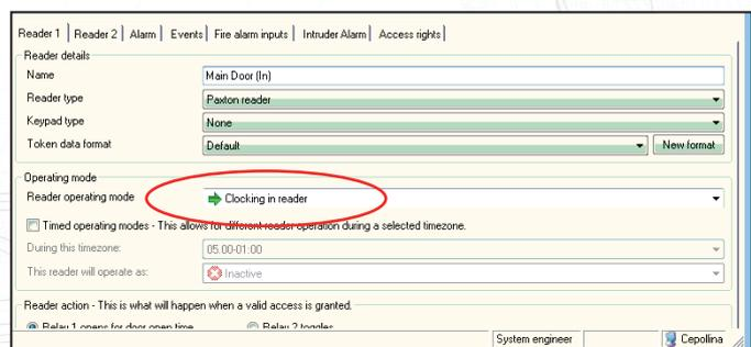
Dedicated readers are required for Clocking In and Clocking Out and cannot be used to control access through a door. Separating these functions ensures accurate time and attendance information.
