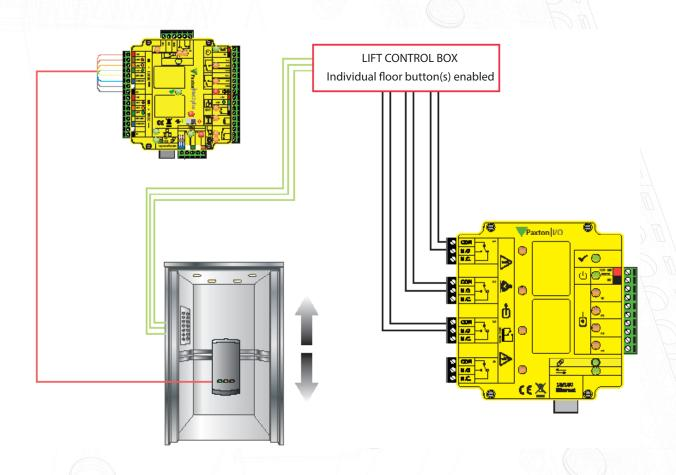
The I/O boards must be set up and configured before appropriate Triggers and Action rules can be set up. A rule must be set up for each floor grouping that you require. (All floors, 1st floor only, etc)
