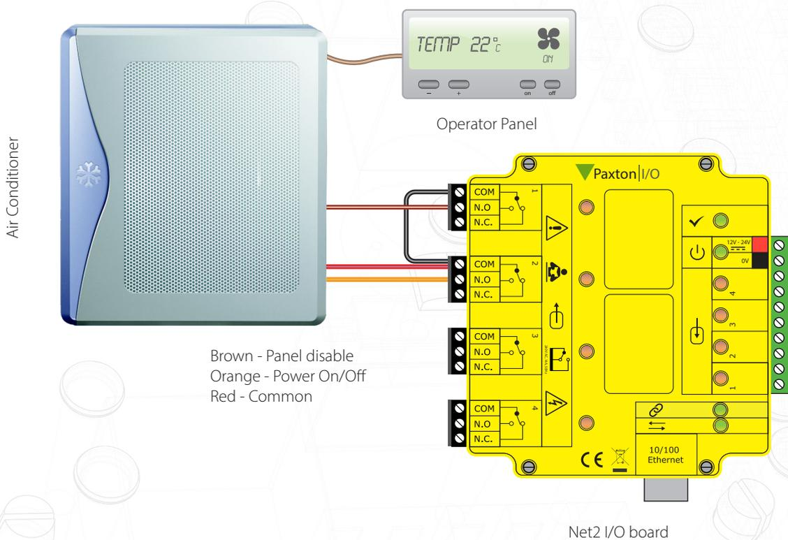
Many air conditioning units have an external interface. In this example we must first disable the operator panel by linking the Red and Brown wires and then break any link between the Red and Orange wires to turn off the unit. Many other options exist depending on your manufacturer but the principles explained here are the same.
