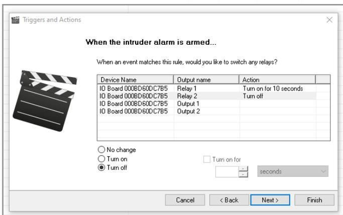
Turn on Relay 1 to disable the operator panel for 10 seconds.
