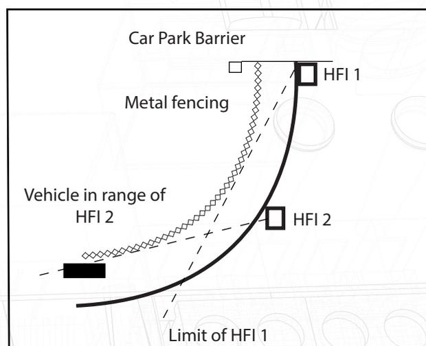
Connecting one ACU port to several interfaces wired in parallel allows them to be positioned along an approaching driveway. The total ACU reader port load should not exceed 500 mA.
