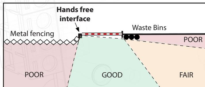
In the above diagram, we have a metal fence alongside the entrance. This will shield the interface from any user approaching from the left.
