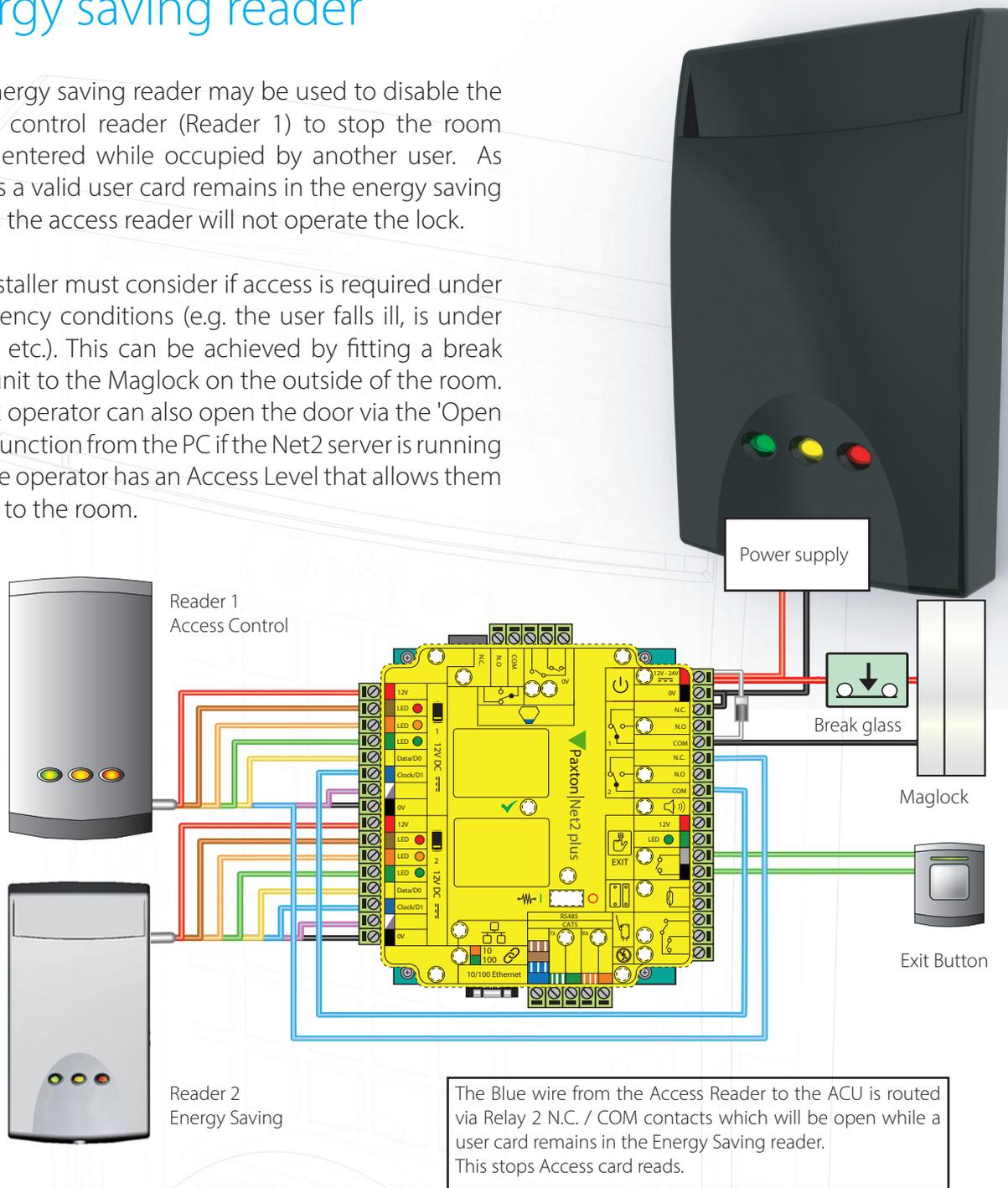
Wire the ACU as per a normal Maglock. As advised above, the 12V feed passes through an external break glass so that the lock can be released from the outside in an emergency.
