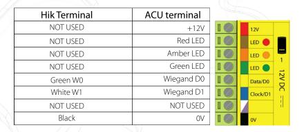
Ensure any unused wires are safely terminated.
