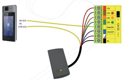
The default door open time on the HIK terminal is 5 seconds. To allow sufficient time for the user to present their token to the Paxton reader, you may wish to increase this via the ACS menu on the HIK terminal.
