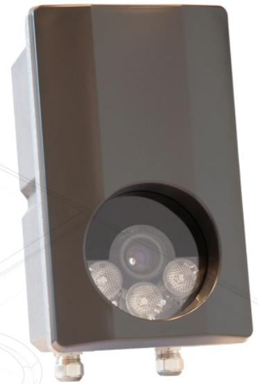
The reader is a self contained unit running on 24V DC. A Wiegand interface module provides Net2 with a 26 bit Wiegand output that is compatible with the Net2 ANPR settings.
