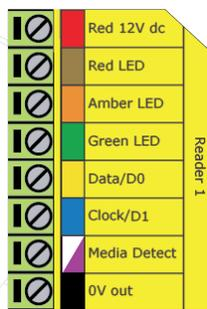
Ensure any unused wires are safely terminated.
