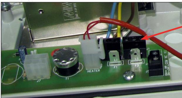
Connect the AC mains supply with Earth wire to the terminal block
